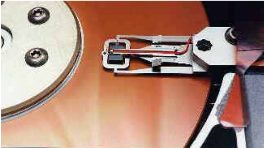
Head assembly of ST412 Drive (10MB drive)
