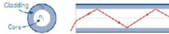
Fig. 1: Optical fiber. The refractive index of the core is slightly higher than that of the cladding. Typical dimensions are 10 or 50 micrometers for the core and 125 micrometers for the fiber. In addition, a protecting plastic "buffer" is placed around the fiber.
